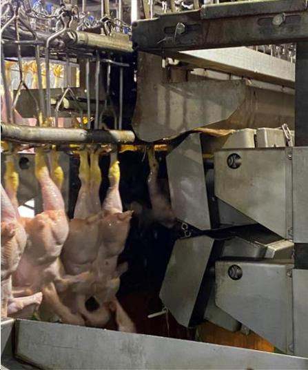
A photograph showing several chickens suspended by their feet on a metal conveyor belt. They are moving through a large industrial plucking machine with various rollers and blades. The scene is brightly lit, and the machinery is metallic and complex. |
