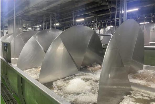
A photograph showing chickens in a large industrial cooling tank. The tank is filled with water, and several large, curved metal blades are visible, likely used for agitating the water. The scene is dimly lit, with some overhead lights.             |
